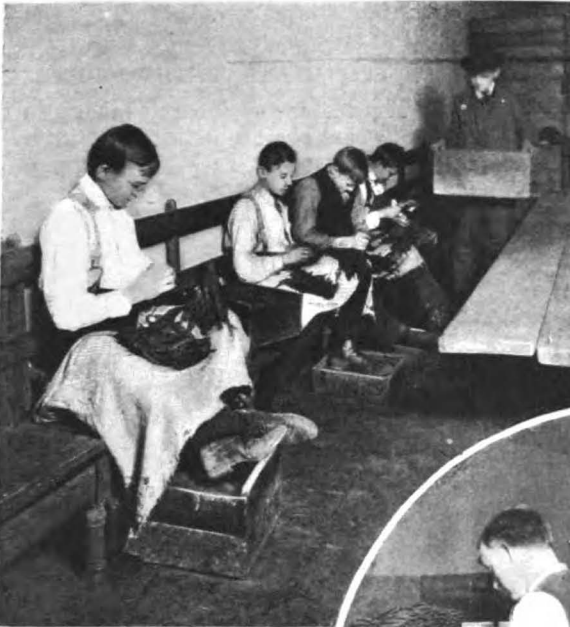
"STRIPPING" TOBACCO—IN THIS PROCESS THE COARSE VEINS ARE REMOVED FROM THE LEAVES.
